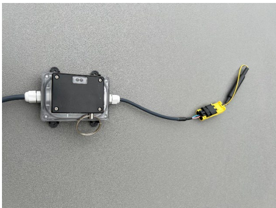
MTS with the test harness connected
