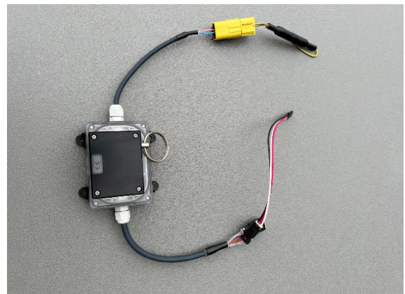
MTS with test harness and wiring connector
