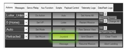
In the joystick window, select the hand controller from the dropdown. On most windows machines, this will be labeled "SRC Application." It will be necessary to map RC1 through RC4, by selecting "Detect" for each one, pressing Okay, then moving the corresponding stick.
